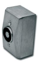
The LCN SEM7800 Series are heavy duty, electrically controlled door holding magnets. Magnets are fail safe and hold until the current is interrupted. A manual door closer is used to control and close the door. A choice of floor, recessed wall, or surface mounted wall magnets are available.
